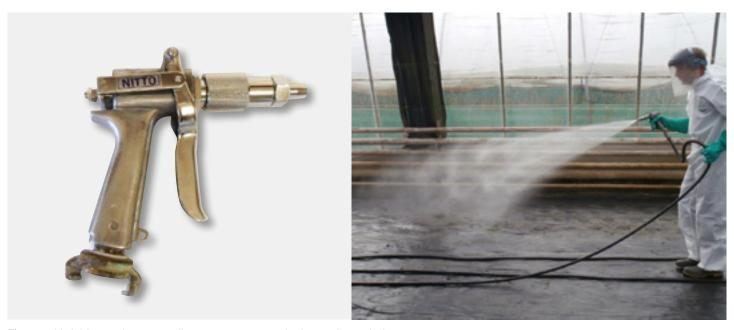
Figure 6. Variable nozzle type applicators are common in the cut flower industry
